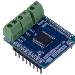
DC Motor Controller
