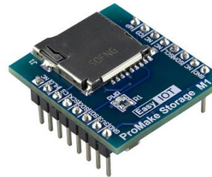
Storage M1 Micro SD Data Logger
