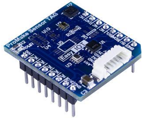
Sensor TAG Temperature, humidity, Light,..
